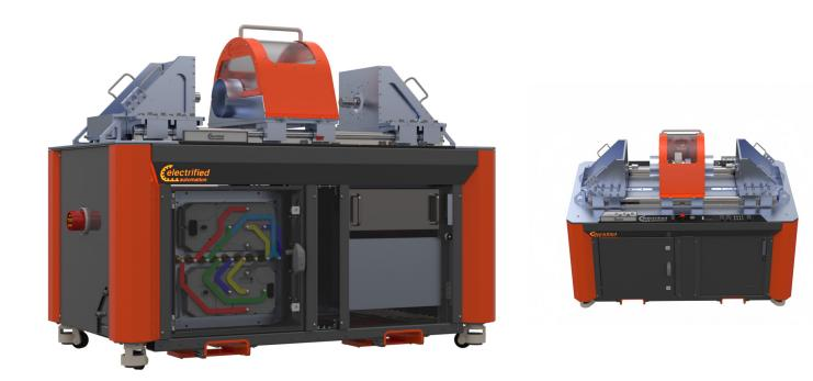
**Rig Dimensions:** 1800mm x 1400mm x 1000mm **Driveline Height:** 1113mm at rotational axle centreline Max Motor Diameter: 315mm Steel Shaft: 40mm diameter & 1500mm length
